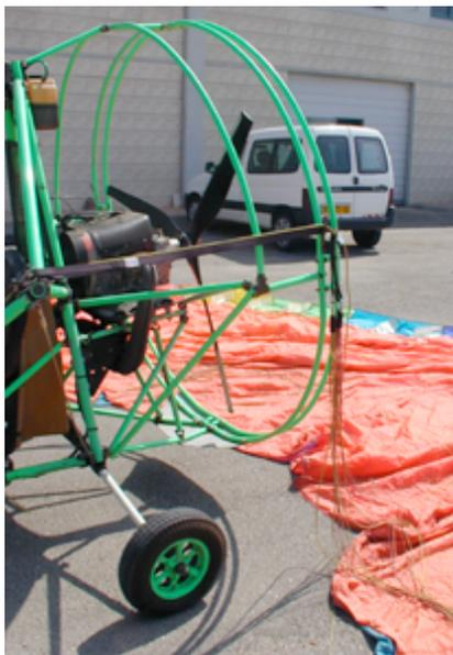
8. Take the main brake line and wrap it 3-4 times to the rest of the lines, make sure not to wrap the risers or the carabiners.
