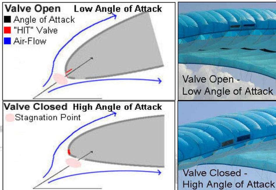
The NRG is equipped with an Active HIT Valve system (patent pending) to improve the overall performance and safety of the wing especially during accelerated flight.
