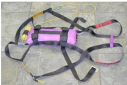
Lay the High-Rise Rescue Chute out on the ground with the parachute container facing down and the harness straps opened as shown.
