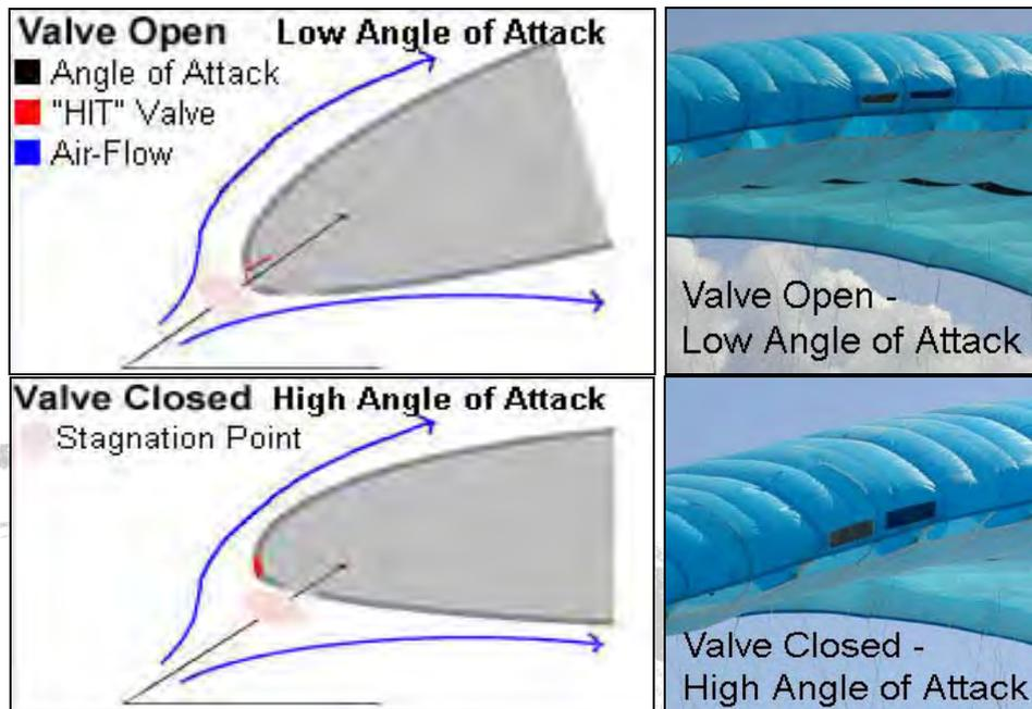
The FORCE is equipped with an Active HIT Valve system (patent pending) to improve the overall performance and safety of the wing especially during accelerated flight.
