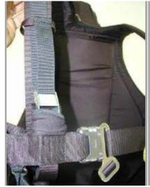
**1.** The **Shoulder Strap** Adjusters are similar to most Apco Harnesses, differing only in the minor improvement, which prevents the free ends of the adjustment webbing from flapping around in the wind. These straps are best adjusted when standing with the chest/leg straps closed. Tighten the shoulder straps so that they are tight while standing upright. While in flight it is normal for these straps to be a little slack.
