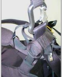
**2.** The **Back/Side Strap** Adjusters these are similar to previous Apco Harnesses. They are best adjusted while the harness is suspended from a suitable structure, before the first flight is made.
