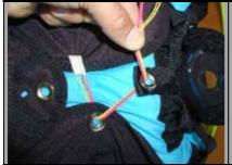
Next close flap No.3 over flaps No.2 and No.1, and thread the pull cords through the grommet attached to the webbing under flap No.3.
