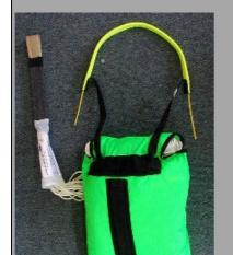
Your harness is supplied with a deployment handle fitted in the correct way. Remove the handle by pulling it out of the elastic retainers. Attach the handle to the deployment bag (44120T) supplied with your <a href="Mayday">Mayday</a> reserve parachute. If your Reserve is not already fitted inside the deployment bag, follow the instructions for doing this on the <a href="Mayday">Mayday</a> page.
