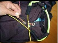
Fit the deployment handle to flap No.4 by pushing its ends (cable first) into the elasticized sleeves with the cables protruding on the other side. The webbing part of the handles should be pushed almost all the way into the elasticized sleeves (stop about 8-10mm before the opening where the cable is protruding).
