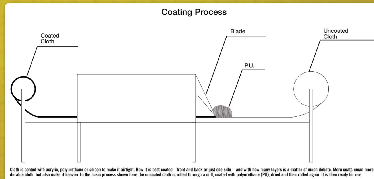
Cloth is coated with acrylic, polyurethane or silicon to make it airtight. How it is best coated - front and back or just one side – and with how many layers is a matter of much debate. More coats mean more durable cloth, but also make it heavier. In the basic process shown here the uncoated cloth is rolled through a mill, coated with polyurethane (PU), dried and then rolled again. It is then ready for use.
