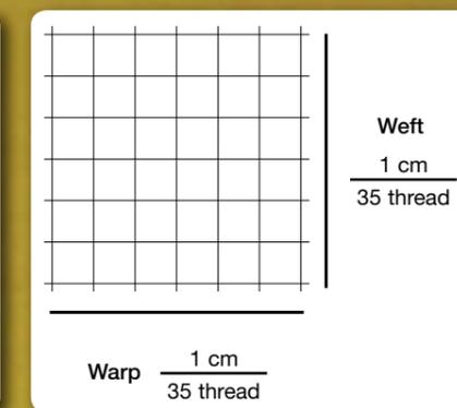
The weight of cloth depends on how tightly woven it is. Industry standard is 50 x 50 threads. To make cloth lighter cloth manufacturers simply use less thread – 40 x 40 is common and 35 x 35 is used for some lightweight paragliders.
