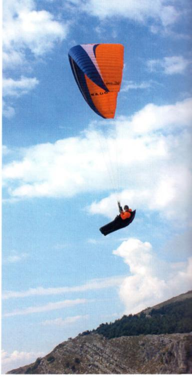
"While the wing is scaled many of the other parameters and forces, such as pilot drag, line diameters etc are not scaled. This means when a wing is zoomed it can be difficult repeating handling and safety of the wing in all sizes."
