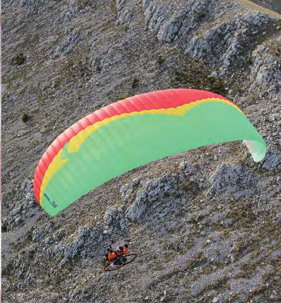
The wing is made from Gelvenor cloth with a silicone coating on the front half. This should mean the wing stands up well to general use and being dragged around as you hone your ground-handling skills. All the lines are sheathed, which makes for easy handling on the ground and in the air. They are all nicely colour-coded too, making it easier to find the line you want.
