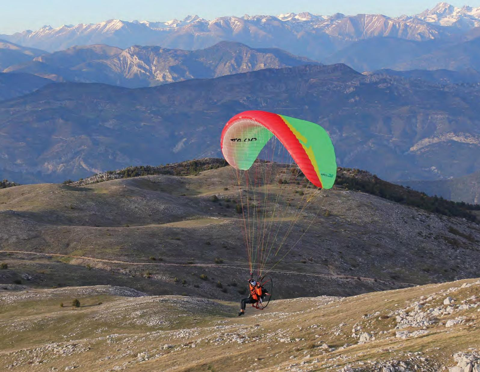
when flying fast: I was able to maintain level flight without having to use full throttle despite the altitude, making it an efficient wing for cross-country tours. As with some other reflex designs the company advise against using the speedbar unless the trimmers are fully open. When flying trimmers-open it is advised that pilots don't use the brakes – use the tip-steering toggles instead.
